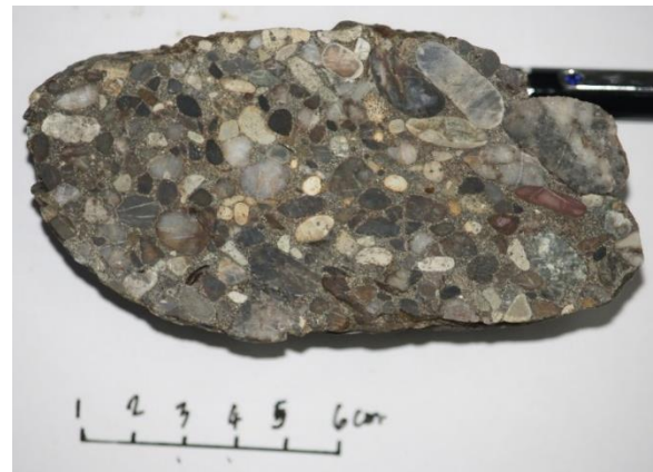
Figure 8. The grab sample of conglomerate with rounded clast of sandstone, slate and quartz.
